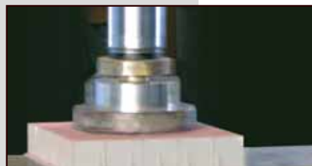
Certified load resistance (more than 203 kn = 20,3 t)*
